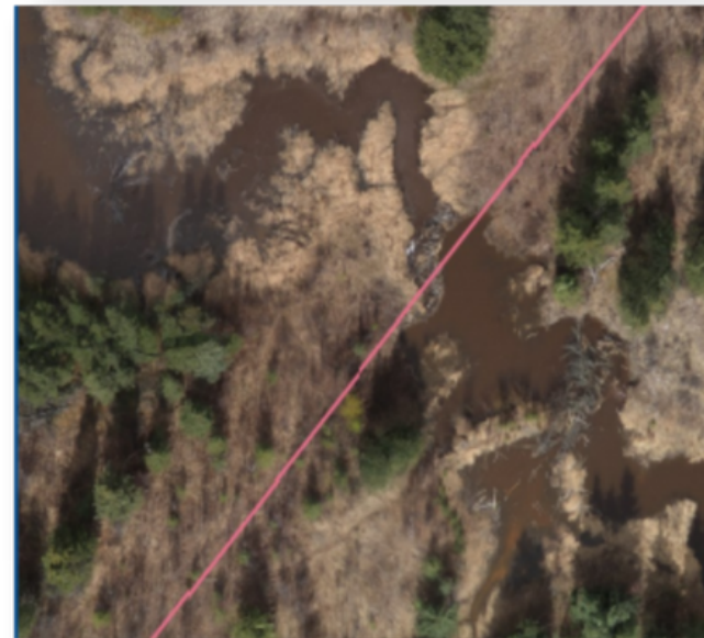
Comparison of Satellite Imagery vs Data Collection During Pipeline Inspection (High Risk Beaver Dam Identified)
